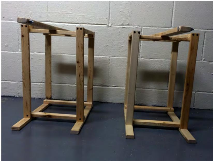
Ryan Williams and I built user testing stands, or tripods with an extended arm to mount a camera. Our purpose for this was to create something that was unobtrusive so that during user testing the angle of the video was directly above the device that the user was testing on. It was important for the camera and the testing stand to be out of the way of the user, so to not cause an uncomfortable experience and still capture what was happening on the screen.
